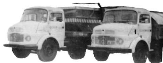
Mod. KPG-90/230-SM-V3 - cap. 9 ton, com caçamba semi-fechada KEDLU-230/70-5-SF - cap. 7,5 m 3
